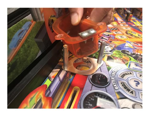
**Step 6.)** Place a washer over the slot in the orange ramp and then fasten the screw back into the hex post, using your #2 Phillips screwdriver. Repeat this step for the other slot in the orange ramp exit. Make sure the fasteners are secure, but do not overtighten.
