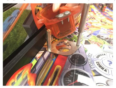
**Step 5.)** Carefully align the Ramp so the slots in each side of the ramp line up with the holes in the hex spacers.
