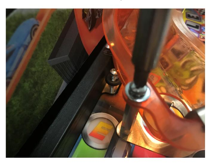
This is how the Ramp Exit Plate should look when installed from the top-down view.
